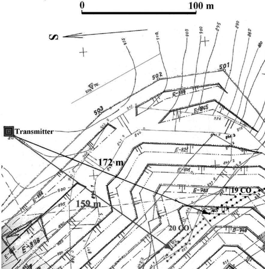
Fig. 2. Position of CO 19 and CO 20 with respect to the transmitter with distances marked in Dubina quarry
