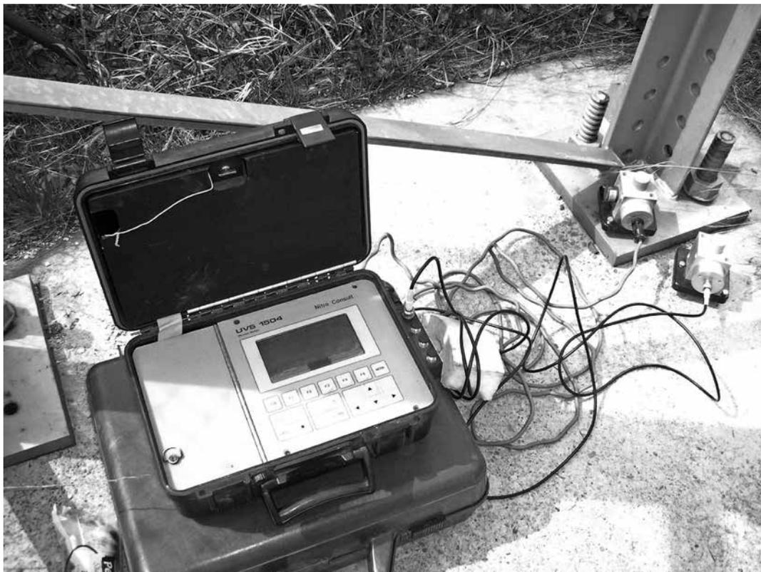
**Fig. 1.** Installation of seismograph and seismic detectors before rock blast on the steel construction of transmitter
