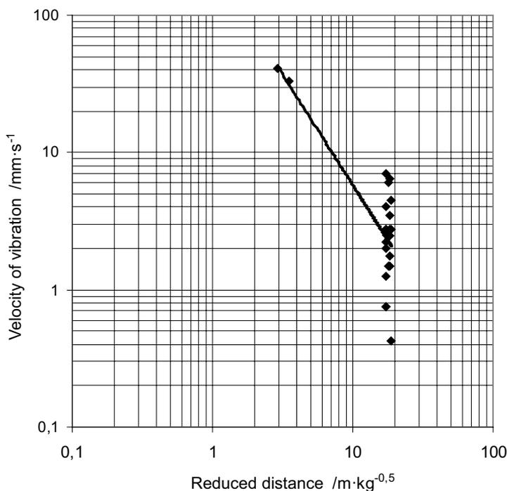
**Fig. 3.** Graphical dependence of maximum component of velocity of vibration on reduced distance for bench blastings in Dubina quarry-the seismic waves' attenuation law
