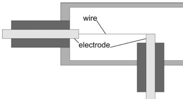
**Fig. 2.** The schematic view of current injection device
