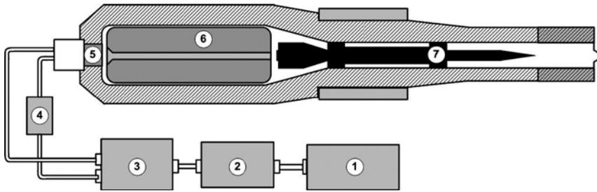
**Fig. 1.** Concept art of an ETC gun [3]: 1) Primary storage; 2) Secondary storage; 3) Pulse forming network; 4) Firing switch; 5) Plasma cartridge; 6) Propellant; 7) Projectile
