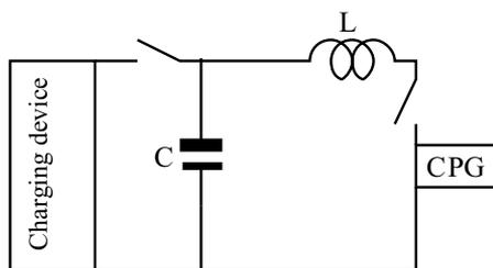
**Fig. 4.** Scheme of Pulse Forming Network with CPG
