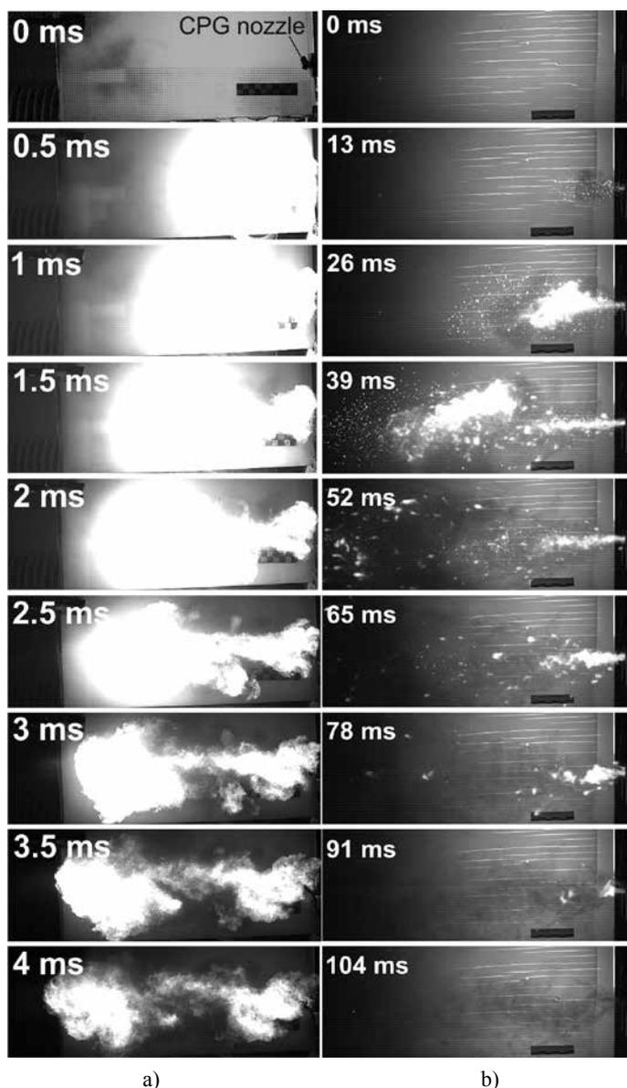
Fig. 5. Plasma (a) and black powder (b) effect of ignition – comparable investigations
