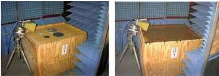
Fig 10. The experiment arrangement. Left: mine surrogates are lying on the sand's surface. Right: minelike targets are embedded and the surface is covered by photothermal film. [10]
