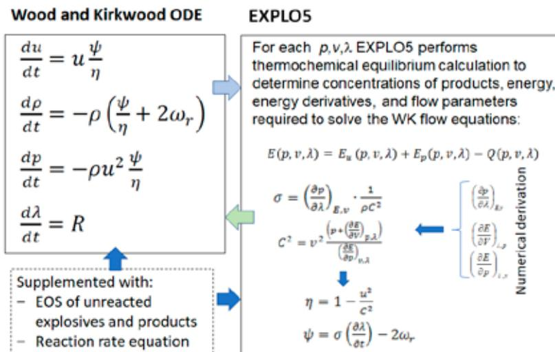
**Figure 2.** Schematic presentation of the model [17]
