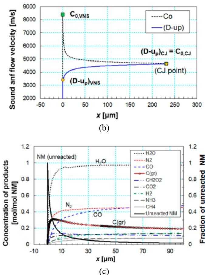
**Figure 8.** Spatial distribution of pressure and temperature (a), sound and flow velocity (b), and concentration of products within first 100  $\mu\text{m}$  ns (25) behind the shock (c); calculation done using PB-C1.7D2 rate model
