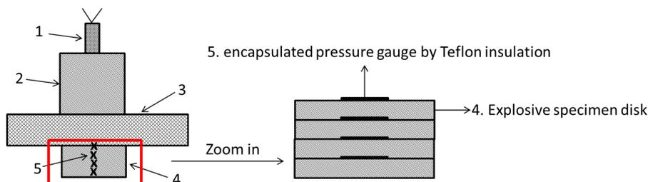
**Figure 1.** A schematic diagram of the shock ignition and growth arrangement for HMX-based PBXs at different temperatures: 1) detonator; 2) primary explosive; 3) aluminum plate; 4) explosive specimen disk; 5) encapsulated pressure gauge with Teflon<sup>®</sup> insulation
