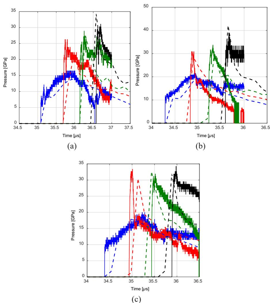
**Figure 4.** Comparison between the experimental (solid lines) and the simulation (dashed lines) results for distances 0 mm (blue), 3 mm (red), 6 mm (green) and 9 mm (black), under different temperature conditions: (a) 25 °C; (b) 80 °C; (c) 120 °C
