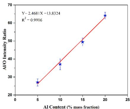
**Figure 7.** Calibration curve using Al/O intensity ratio versus Al content of the TNT/Al standard samples in an Ar atmosphere
