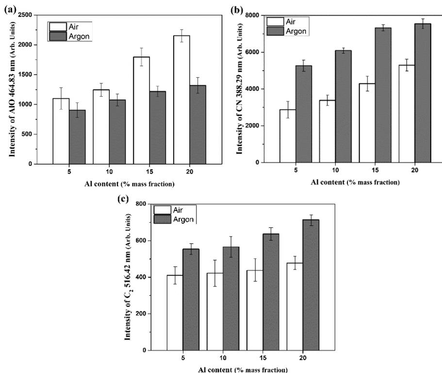
**Figure 2.** Bar diagrams of (a) AIO (464.83 nm), (b) CN (388.29 nm), (c) C<sub>2</sub> (516.42 nm); intensities versus Al content in TNT/Al standard samples for comparison intensities, in two atmospheres (air and Ar)
