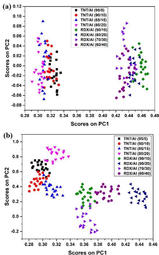
**Figure 3.** Two-dimensional PCA scores for aluminized TNT and aluminized RDX samples in two atmospheres: (a) air and (b) Ar
