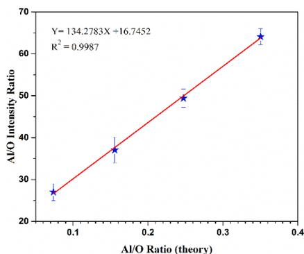
**Figure 4.** The measured Al/O intensity ratio by LIBS in an Ar atmosphere versus the Al/O composition ratio of TNT/Al given in Table 2
