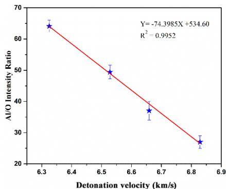
**Figure 5.** Al/O intensity ratio versus detonation velocity in the TNT/Al standard samples
