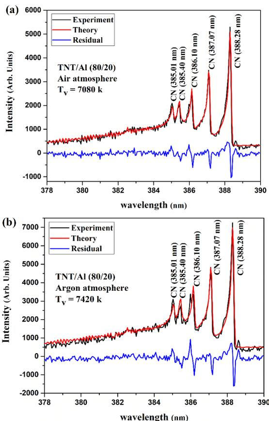
**Figure 8.** Comparisons between experimental and theoretical spectra, which were obtained using a NMT program for CN violet from LIB spectra of TNT/Al (80/20) standard sample of the sequence  $\Delta\nu = 0$ , in two atmospheres (a) air (b) Ar
