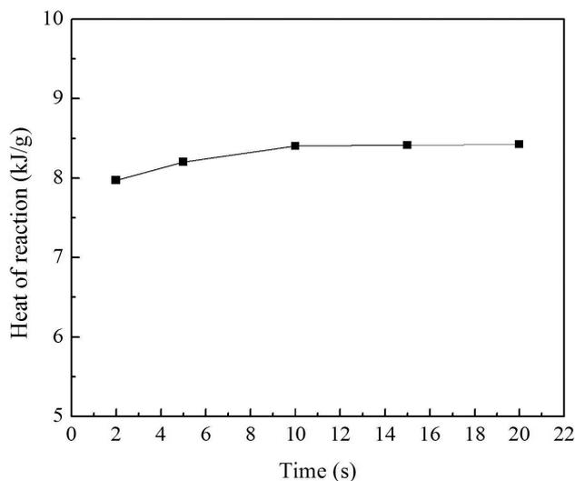
**Figure 4.** The heat of reaction for a PTFE/26.5 wt.% Al composite at different laser irradiation times but the same laser power level of 18 W
