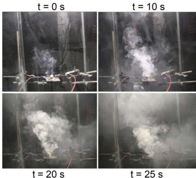
**Figure 1.** Burning of a 2 g pellet of formulation 4
