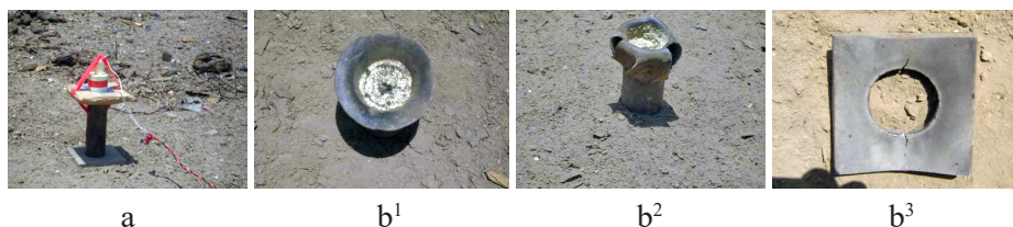
Figure 3. Shock sensitivity test of a DNAN charge: (a) test arrangement; (b) test results: 5.5 GPa (b 1 ), 5.8 GPa (b 2 ), 6.0 GPa (b 3 )
