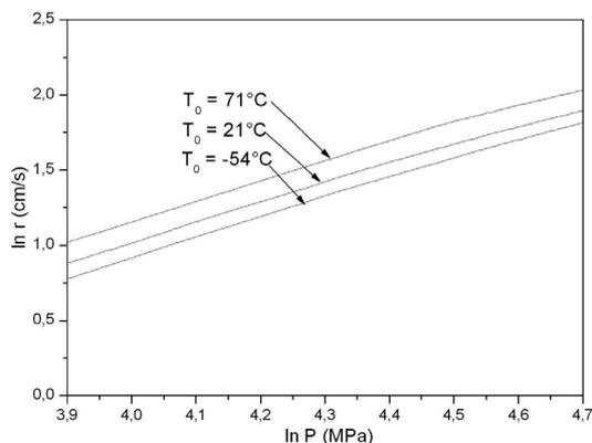
**Figure 1.** Temperature dependence of the burning rate for the spherical single base propellant [11]
