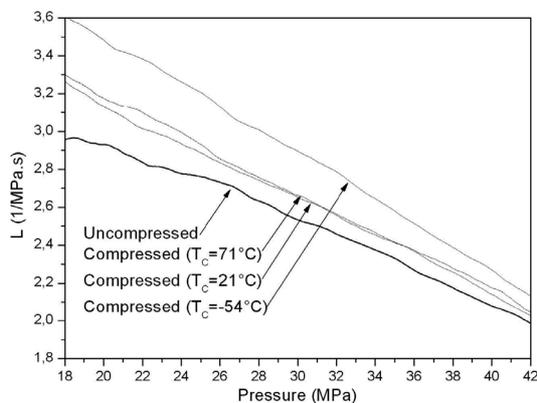
**Figure 7.** The dynamic vivacity of the uncompressed propellant tested at  $T_0 = 21\text{ }^\circ\text{C}$  (benchmark) and the compressed propellant at various initial temperatures ( $T_c$ )
