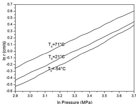
**Figure 3.** Temperature dependence of the burning rate for the spherical single base propellant
