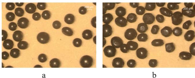
**Figure 6.** Photomicroscopy of (a) the spherical propellant grains, and (b) grains from the compressed propellant bed
