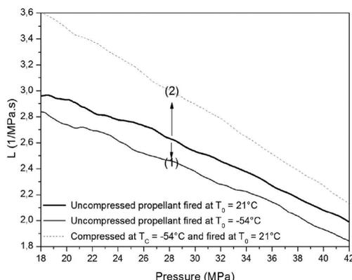
**Figure 8.** Effects on the dynamic vivacity: (1) decrease of the initial temperature, and (2) compression at  $-54\text{ }^{\circ}\text{C}$
