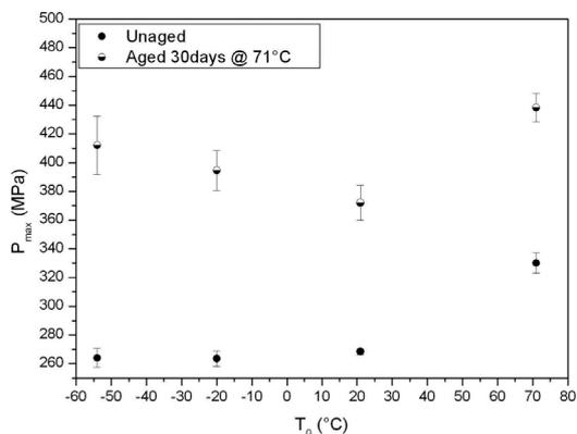
**Figure 2.** Variation of the maximal pressure inside the cartridge as a function of the initial temperature of the unaged and aged (30 days at 71 °C) propellant (10 shots), the displayed error bars are  $\pm 1$  standard deviation (SD)
