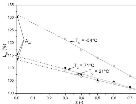
**Figure 9.** Relative vivacity as a function of the burn fraction at various initial temperatures ( $T_c$ )
