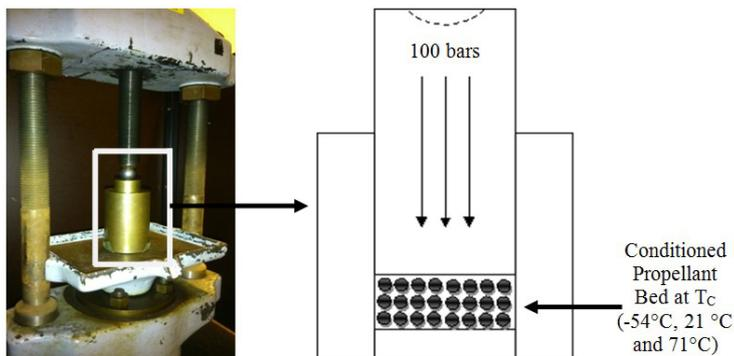
**Figure 5.** Compression of the conditioned propellant beds ( $T_C$ ) at a pressure of 100 bar for 1 min using a manual hydraulic press. The conditioning temperatures ( $T_C$ ) were equal to  $-54\text{ }^\circ\text{C}$ ,  $21\text{ }^\circ\text{C}$  and  $71\text{ }^\circ\text{C}$ . The mass of the propellant bed was 1 g
