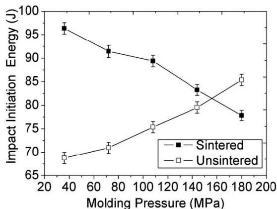
**Figure 7.** Plot of impact initiation energy of sintered and unsintered Al-PTFE against molding pressure (data points are average values from 25 independent tests  $\pm$  the standard deviation).
