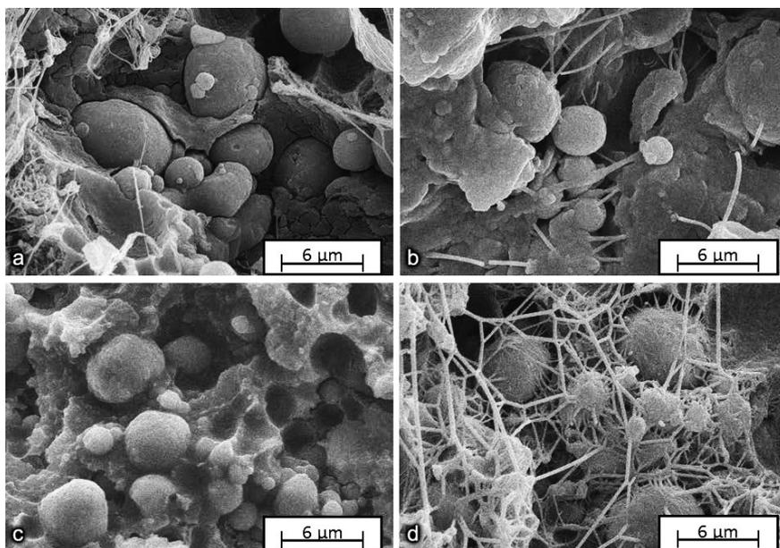
**Figure 5.** SEM images of the interior microstructures of Al-PTFE produced by different processing procedures: (a) unsintered Al-PTFE pressed under 36 MPa; (b) unsintered Al-PTFE pressed under 182 MPa; (c) sintered Al-PTFE pressed under 36 MPa; (d) sintered Al-PTFE pressed under 182 MPa.
