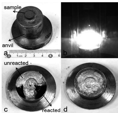
**Figure 6.** Impact initiated reaction of Al-PTFE in drop-weight test: (a) Al-PTFE sample placed on the anvil before the drop-weight test, (b) flame captured by high speed photography in the drop-weight test, (c) reacted Al-PTFE after a drop-weight test, (d) unreacted Al-PTFE after a drop-weight test.
