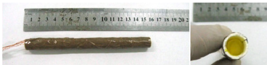
Figure 5. Explosive charge prepared for detonation velocity determination.
