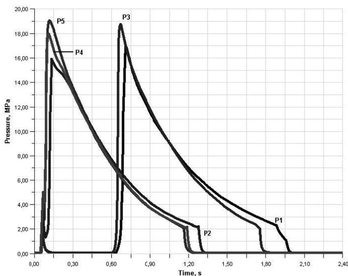
**Figure 4.**  $p = f(t)$  curves for the propellants examined.
