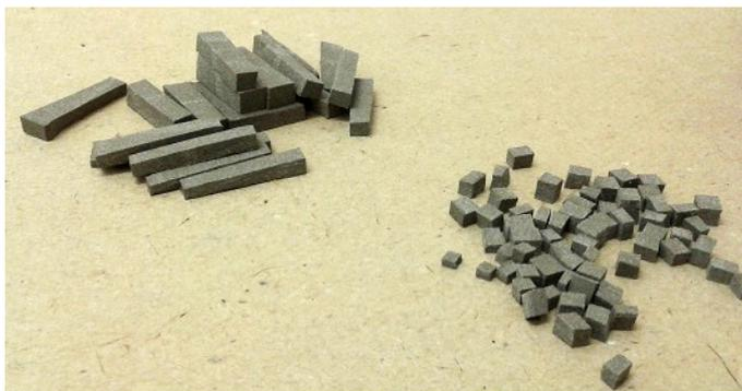
**Figure 1.** A sample of the shredded propellant.
