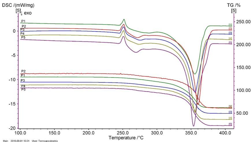
**Figure 3.** DSC/TG curves of the propellants examined.
