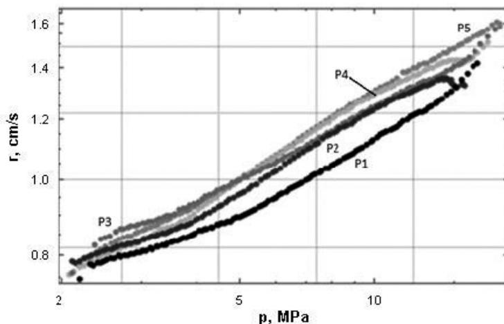
**Figure 5.** Dependence of  $r=f(p)$  for the propellants examined.
