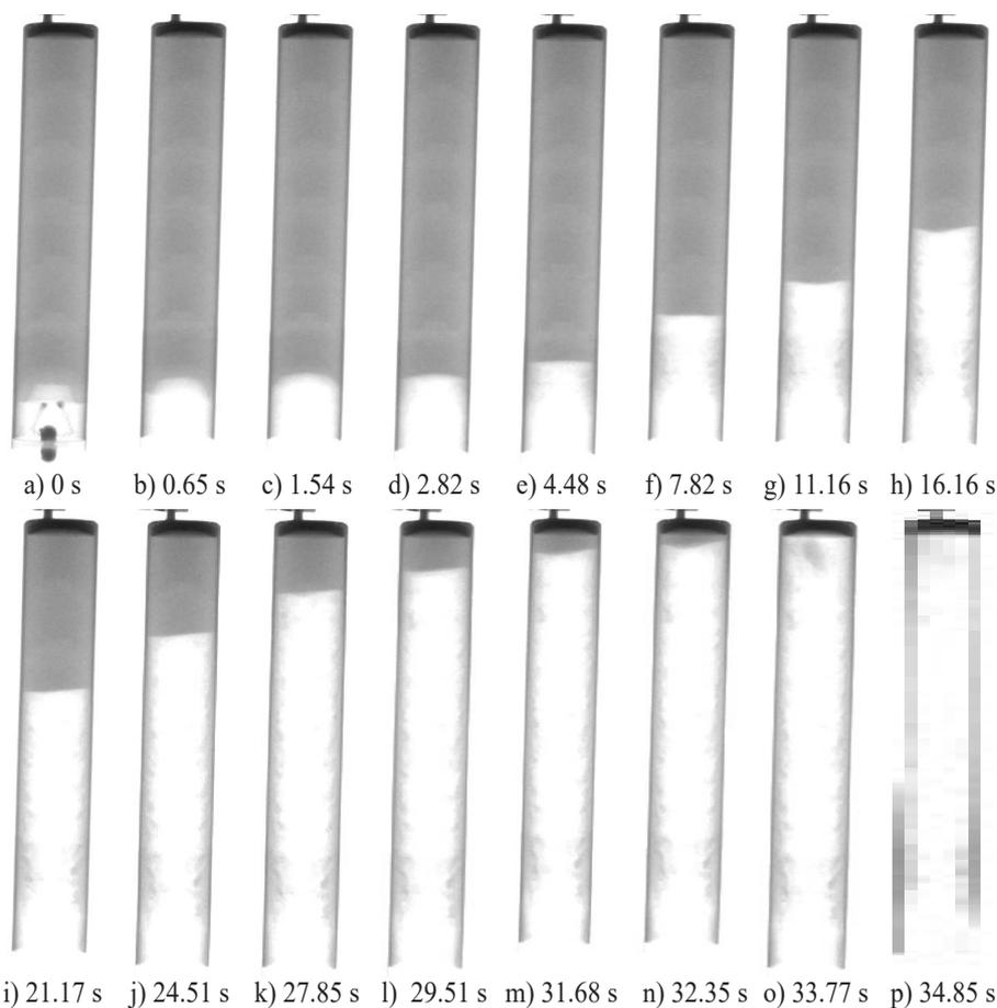
**Figure 4.** Sequence of RTR images of the tested anti-tank missile tracer just before its ignition and then during its combustion. Time points of each frame, are shown below each image.
