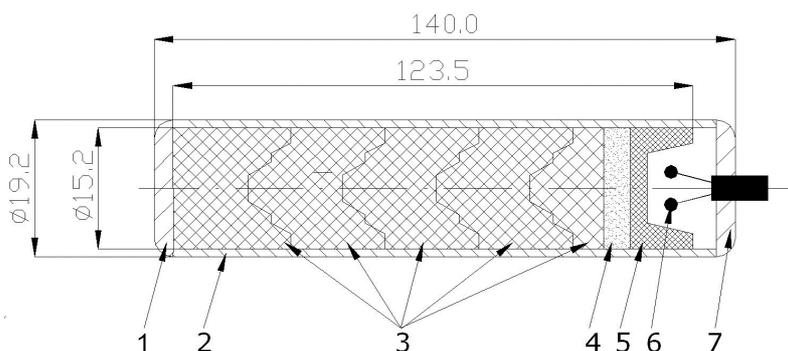
**Figure 2.** Axial cross-sectional view of the anti-tank guided missile tracer: 1) Forward plastic disc; 2) Steel body; 3) Main tracing pyrotechnic elements (segments); 4) Intermediate pyrotechnic segment; 5) Input ignition increment with cavity of trapezium-shaped cross-section; 6) Double electric fusehead system; 7) Rear plastic closure. Dimensions are in mm.
