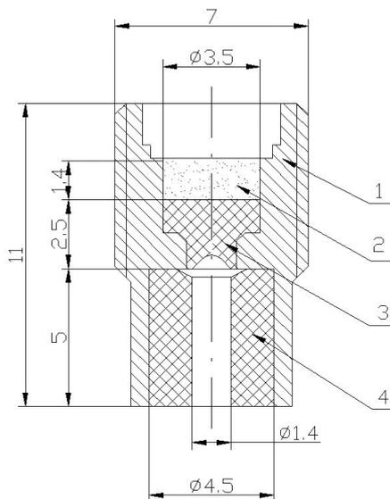
**Figure 1.** Axial cross-sectional view of the delay element used in the RGM type impact artillery fuse: 1) Steel body of the delay element; 2) Input-ignition pyrotechnic increment; 3) Main delay pyrotechnic increment with concave surface; 4) Tubular output ignition augmenting pyrotechnic increment. Dimensions are in mm.
