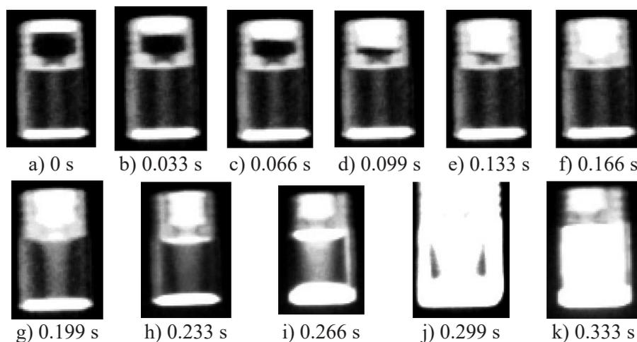
**Figure 3.** Sequence of RTR images of the tested delay element of the RGM type impact artillery fuse just before its ignition, and then during its combustion. Time points of each frame, are shown below each image.
