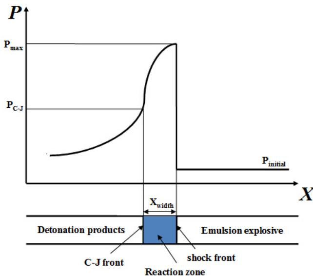
**Figure 4.** Schematic diagram of the ZND detonation model.
