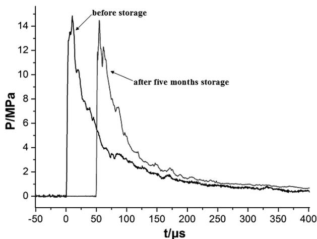
**Figure 2.** Pressure-time curves of the GM-MgH<sub>2</sub> sensitized emulsion explosive, before and after storage.
