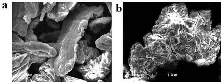
**Figure 1.** Micrograms of MgH<sub>2</sub> powders: (a) untreated; (b) coated with paraffin.
