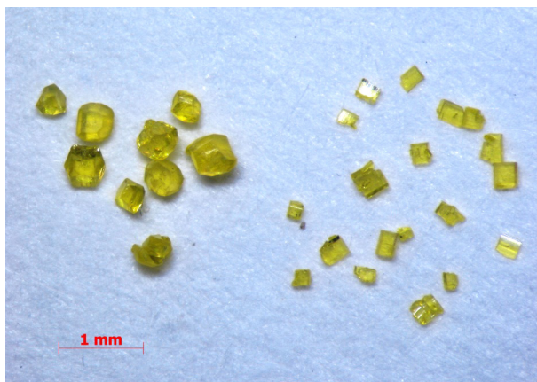
Figure 11. Two kinds of crystals present in the investigated FOX-7 sample.
