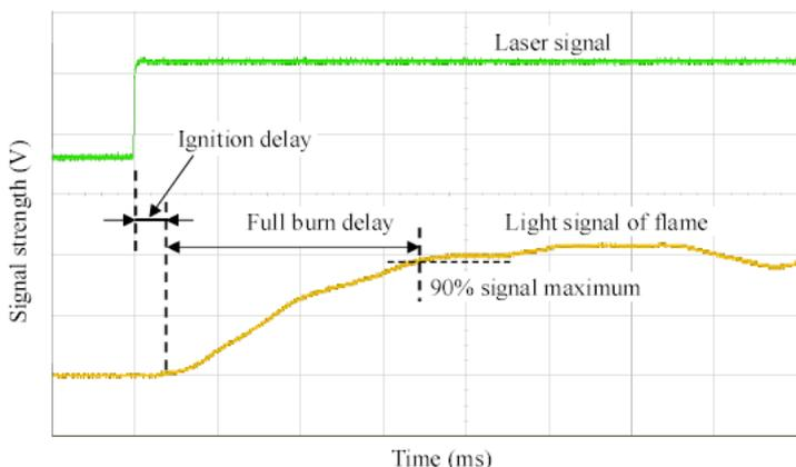
**Figure 5.** Oscilloscope traces illustrating the light signals from the laser and the ignition flame and defining the ignition delay time and the full burn time.
